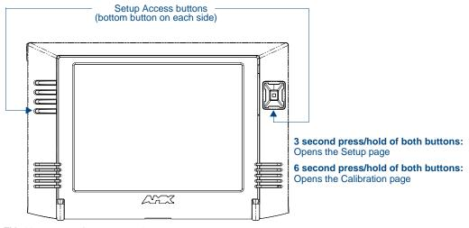
FIG. 88 Location of Setup Access buttons
